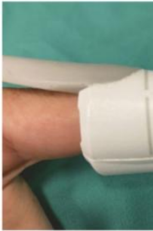
Fig. 1 Sonivate SonicEye® finger sound transducer. The fingertip slides onto a finger.
